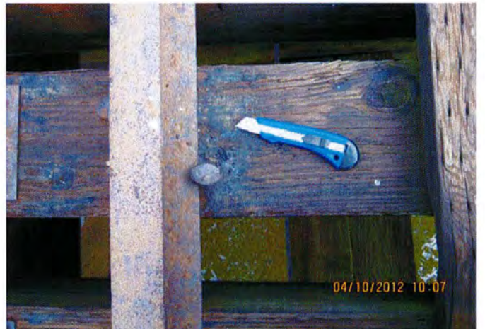
Asbestos Sample 04, oil/coating on north tie PCB Sample 003, oil/coating on north tie
